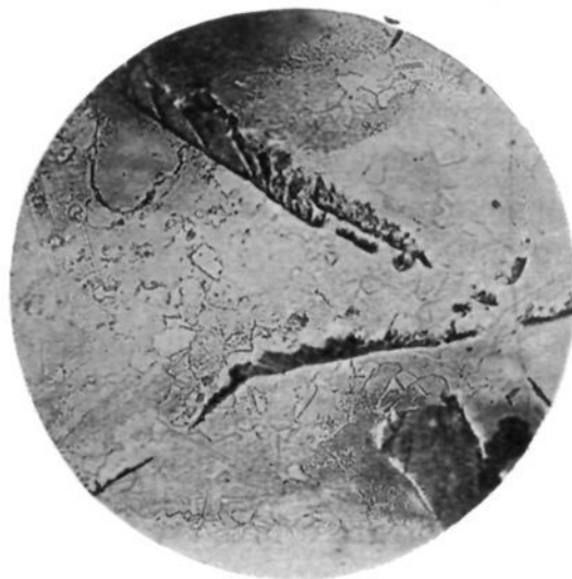
Fig. 5.—98.95% of Pb, 1.0% of Sb, 0.05% of Cu, showing primary blue-violet needles of \text{Cu}_2\text{Sb} .
