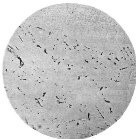
Fig. 4.—99.95% of Pb, 0.05% of Cu, showing needles sticking up from surface.
