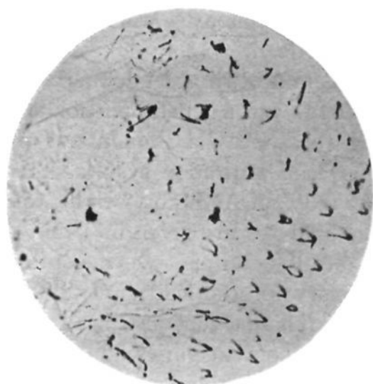
Fig. 3.—99.9% of Pb, 0.05% of Sb, 0.05% of Cu, showing needles sticking up from surface.
